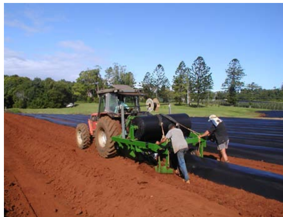
Figure 2. Machines laying plastic mulch and irrigation on mounds.
